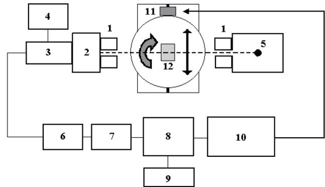
**Figure 2** - Schematic diagram of the first generation tomograph. (1) lead collimators; (2) NaI(Tl) detector; (3) photomultiplier tube; (4) high-voltage unit; (5) <sup>241</sup>Am source; (6) amplifier; (7) monocal analyzer; (8) counter; (9) timer; (10) microcomputer; (11) stepping motor and (12) soil sample. Reprinted, with permission, from Pires *et al.* (2002); copyright Elsevier Science Publishers.
