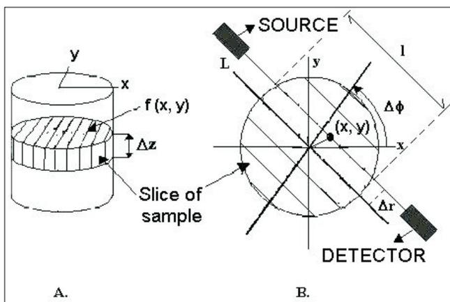
**Figure 1** - Projections from a specific object using computed tomograph. A) Represents the slice of a object defined as  $f(x, y)$  and having a uniform thickness  $\Delta z$ . B) Coordinate system used to describe the tomography image reconstruction method.
