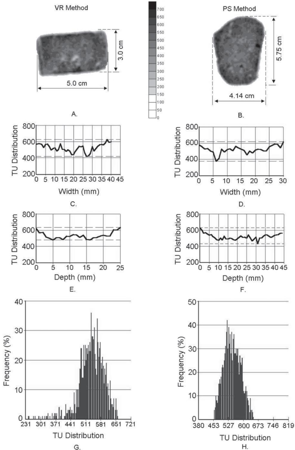
**Figure 4** - (A-B) CT images of soil samples used for analysis of soil density by the volumetric ring (VR) and by the paraffin sealed clod (PS) methods. (C-F) Analysis of transects in width and depth of samples used in the VR and the PS methods. (G-H) TU (Tomographic Unit) distribution histograms obtained for samples collected with volumetric rings and by the PS method.
