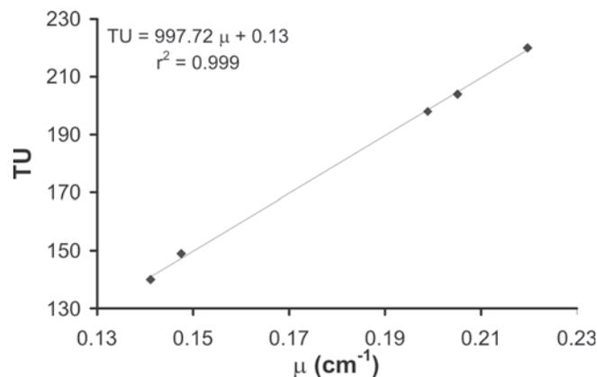
**Figure 3** - CT calibration for  $^{241}\text{Am}$  gamma photons.
