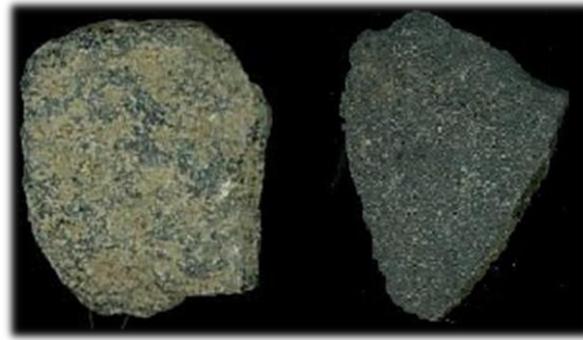
Figure 1: Texture of weathered (left) and non-weathered (right) aggregates samples.
