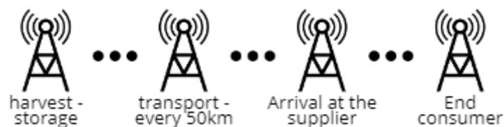
Figure 3. Reading points for the information contained in the RFID Tag.
