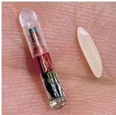
Figure 3 – Chip RFID compared to a grain of rice [14]
