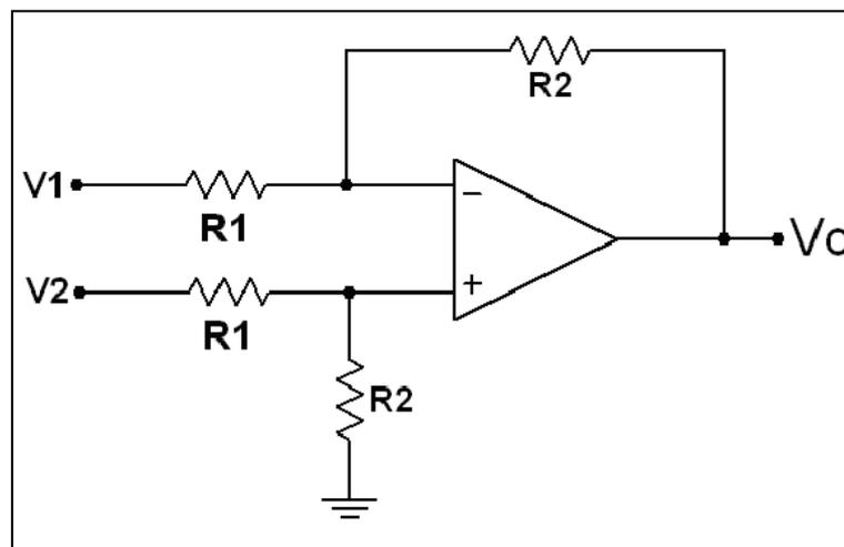
**Figure 3. Circuit in subtractor configuration used in the development of signal suitability system.**
