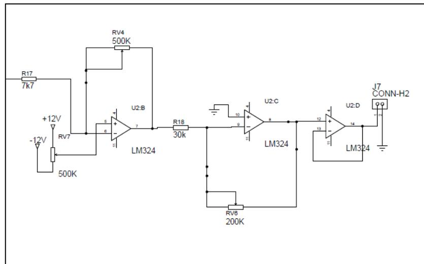
**Figure 4.** Circuit used in the offset, amplification, and connection system in the signal conditioning
