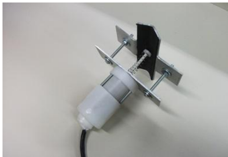
Figure 7: LVDT Sensor constructed in the laboratory
