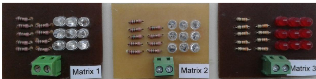
Figure 3. Three different matrixes forming a 3x3 LED matrix.
