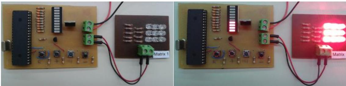
Figure 8. Finalized prototype. On the left side, the system is off, and on the right side, it is working.
