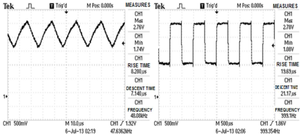
Figure 8 - Received by the photodiode signal with 50KHz and 1KHz
