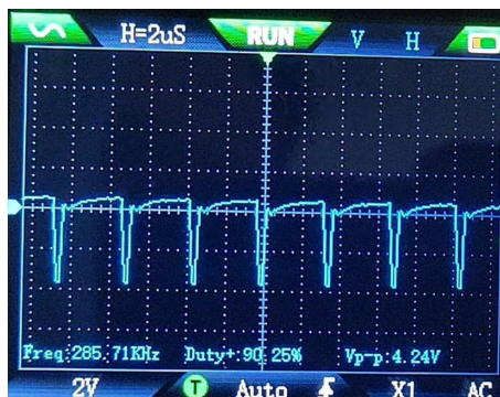
Figure 5: NE555P IC output waveform for pure cachaça sample (100%). Source: The Authors
